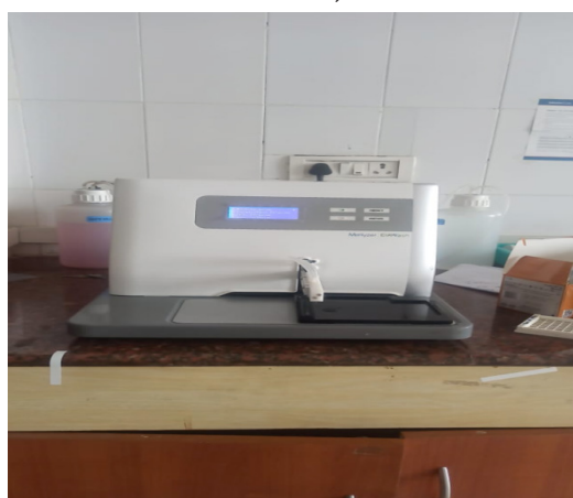
Figure 6: High-sensitivity microplate reader used to measure the optical density (OD) of the ELISA samples for calculating biomarker concentrations (ELISA Reader).
